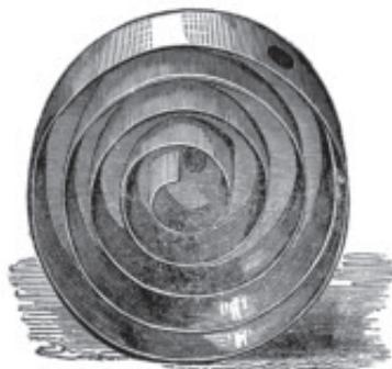
Interior of spiral chamber, the bottom being removed.
